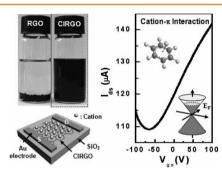
Highly concentrated and conductive reduced graphene oxide (RGO) nanosheets are prepared by introducing monovalent cation– $\pi$  interactions between Na<sup>+</sup> or K<sup>+</sup> ions and six-membered sp<sup>2</sup> carbons on graphene. Current–voltage characteristics demonstrate the interactions in terms of the presence of n-type doping effect due to the adsorption of cations with high electron mobility (39 cm<sup>2</sup> V<sup>-1</sup> s<sup>-1</sup>).
