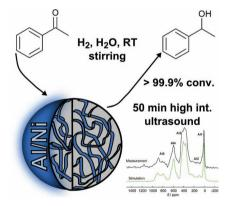
Sonochemical activation of Al/Ni particles results in nanostructuring of initial Al/Ni alloy and the formation of an effective and reusable catalyst for the hydrogenation reactions. This catalyst can be stored and handled under ambient conditions, in comparison to traditional Raney Ni catalysts. The catalyst is fully characterized and catalytic experiments are carried out.
