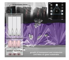
In a race to find alternatives to indiumtin-oxide (ITO) in flat panel display technology, replacement materials are extensively investigated. The basic principles of crystal growth under geometrically constrained conditions are exploited to manufacture highly transparent (82%) and conductive (100  $\Omega$  sq $^{-1}$ ) ZnO films on inexpensive glass substrates.
