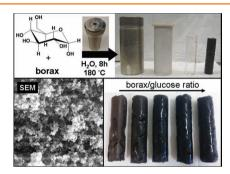
Hierarchically structured carbon aerogels with high surface areas are produced using only glucose as a carbon precursor. A simple, rapid, efficient, and sustainable hydrothermal approach is presented in which sodium borate (borax) is used as a novel catalyst and complex structure directing agent leading to nanostructured, carbonaceous monoliths that are structurally similar to the well-known sol-gel monoliths made of resorcinol and formaldehyde.
