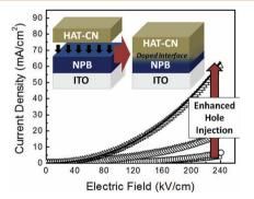
Hole injection is substantially enhanced using 1,4,5,8,9,11-hexaazatriphenylene hexacarbonitrile (HAT-CN) as a hole-injection layer (HIL) with a top anode. The enhanced hole injection is achieved due to the strong electron accepting nature of the hole-transporting layer HAT-CN molecule and efficient doping at the surface of the hole-transporting layer (HTL). The more efficient top injection contact is due to the stronger doping effect of the HIL.
